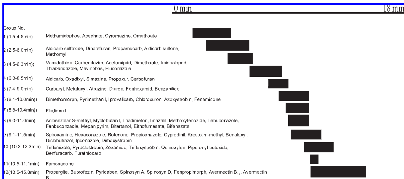
Figure 2. UPLC-MS/MS acquisition sequence of 12 groups used to analyze 72 pesticides, the internal standard (fluconazole), and quality control standard (benzaniide) in the wine.
